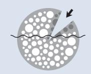
Because the individual air cells are totally enclosed, very little water penetrates. Even if punctured with a through-hole, buoyancy is unaffected and it will not sink.
